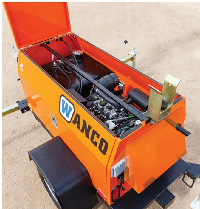
Engine access with maintenance panel raised
